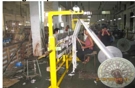
(2) Drawing the warp beam ready for weaving
